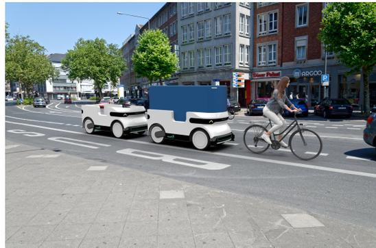
Figure 1.3: Virtual coupling of logistics vehicles [DroidDrive GmbH, 2021b]
