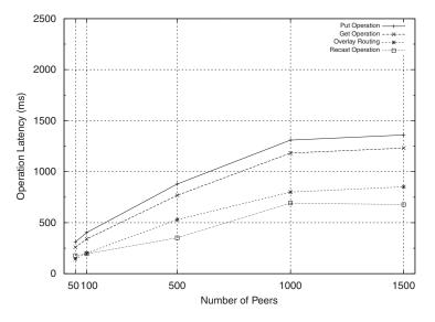
Figure 18. Latency of DhtFlex for mutable data resources.
