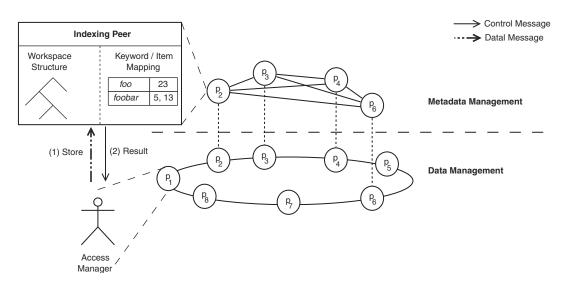
Figure 13. Content data storing in case of a hybrid overlay.
