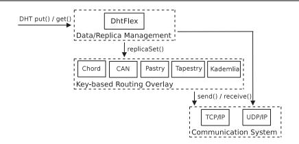
Figure 9. Interactions of the major building blocks of DhtFlex's system environment.
