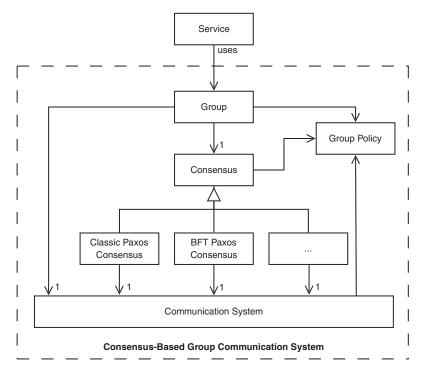
Figure 8. Modular structure of the reconfigurable consensus-based group communication system.
