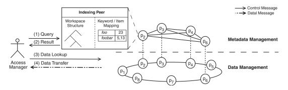
Figure 12. Content data retrieval in case of a hybrid overlay.
